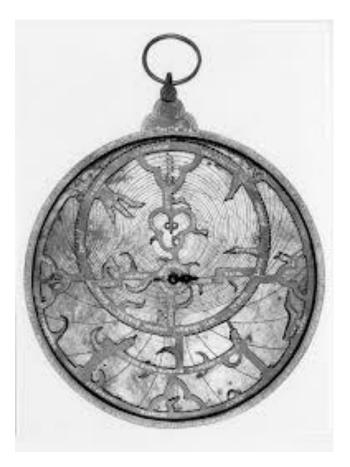
The astrolabe was used by astronomers and navigators to locate the positions of the Sun, Moon, planets, and stars. It was invented by Hipparchus in 150 B.C. and worked similar to a primitive calculator.
